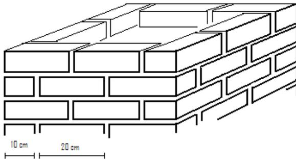
Generally speaking, to be large enough to accommodate nesting or roosting swifts, a chimney should be at least 2 1/2 standard bricks wide on each side.
